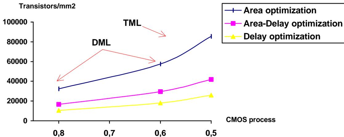
Figure 5 : Densities ( $\text{tr}/\text{mm}^2$ ) for different CMOS processes estimated by equation 1
