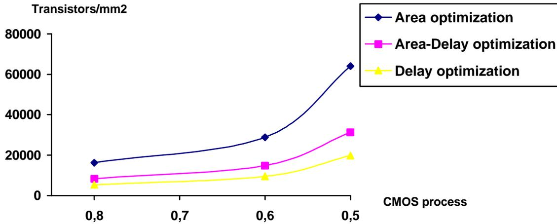
Figure 6 : Densities ( $\text{tr}/\text{mm}^2$ ) for different CMOS processes estimated with routing
