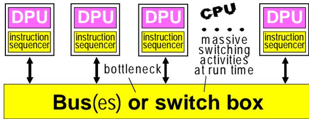
Fig. 7: Typical concurrent computing platform (memory not shown)
