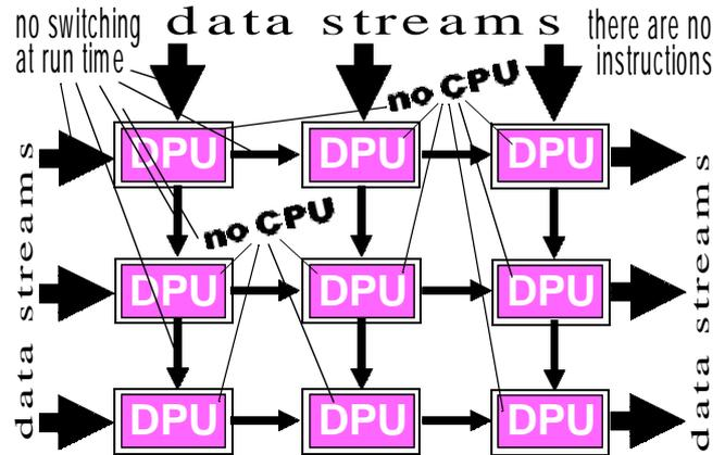
Fig. 8: Stream-based computing array example: transport-triggered exec.
