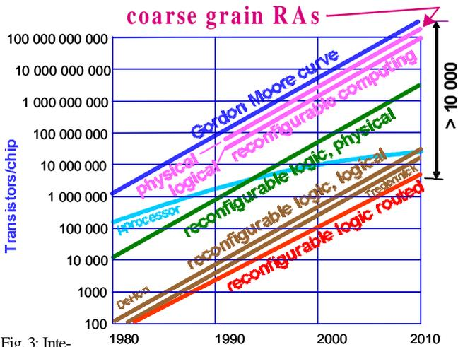
Fig. 3: Integration density of coarse grain reconfigurable computing arrays.
