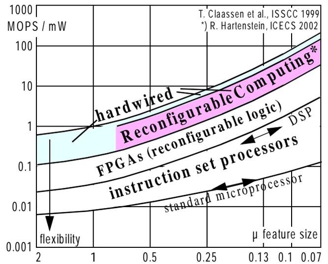
Fig. 4: Energy efficiency vs. flexibility including Reconfigurable computing.
