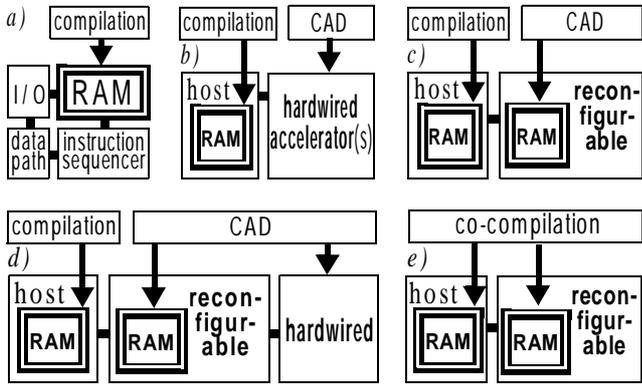
Fig. 11: Computing platforms: a) "von Neumann"-based b) embedded, c) FPGA-based embedded, d) mixed embedded, e) configware / software co-compilation, f) CoDe-X automatically partitioning Co-Compiler.
